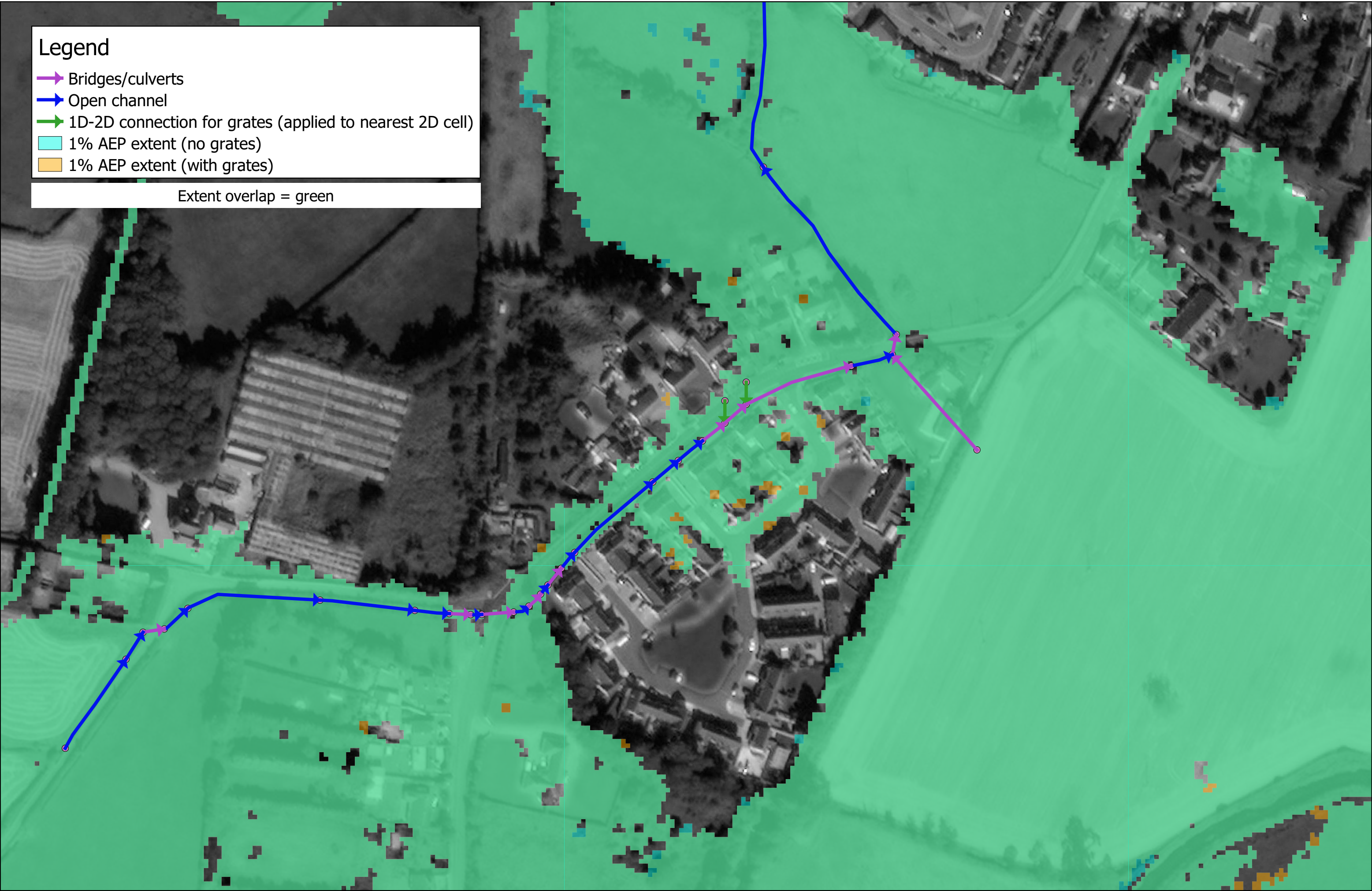
Sensitivity test - inclusion of grates along the Manor Court culvert
